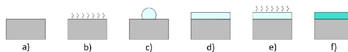
Figure 1.2: Spin-coating: a) the cleaned substrate, b) pre-bake, c) the resist applied in the form of a droplet, d) the resist equally spanned, e) hard-bake, f) the sample is ready for exposure [16].
