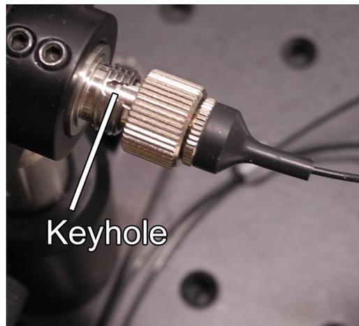
Figure 3: Photo of polarization-maintaining fiber connected to collimator. Connector key fits into keyhole so we have angular position of the fiber under control.
