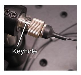
Figure 3: Photo of polarization-maintaining fiber connected to collimator. Connector key fits into keyhole so we have angular position of the fiber under control.
