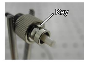
Figure 2: Photo of polarization-maintaining fiber FC/PC connector.
