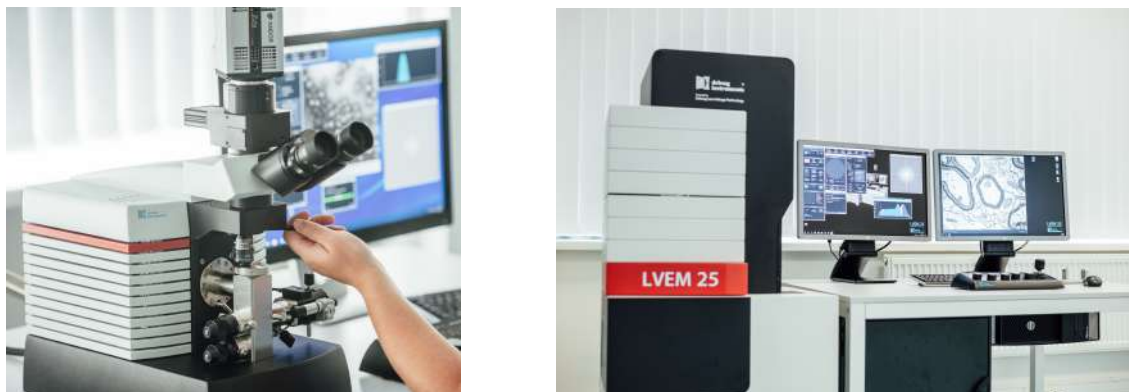
Figure 2.1: The left side shows LVEM5. Its minimal dimensions are clear from the comparison with the operator's hand. The right picture is dedicated to complete workstation of LVEM25.
