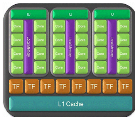
Obrázok 3.7: Detail na Thread Processing Cluster; IU - Instruction Unit, TF - Texture Filter, prevzaté z techreport.com
