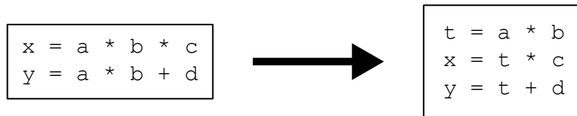
Figure 1.11: Example of common subexpression elimination
