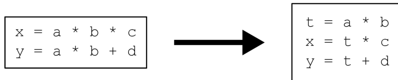
Figure 1.11: Example of common subexpression elimination
