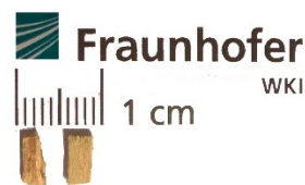
Figure 1. Samples prepared for digital image correlation; particleboard sample – left, MDF sample - right
