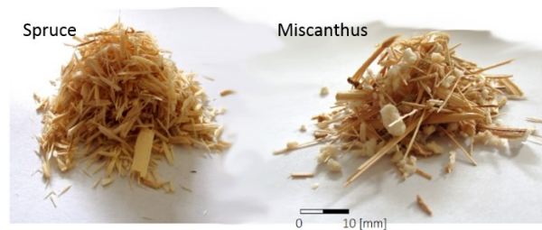
Figure 5-1 Spruce and Miscanthus particles used in production of a particleboard panel
