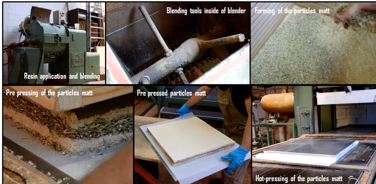
Figure 3-2. Production flow of the particleboard
