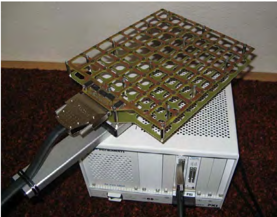
Figure 5.6: Measurement system with matrix microphone array and digital MEMS microphones.
