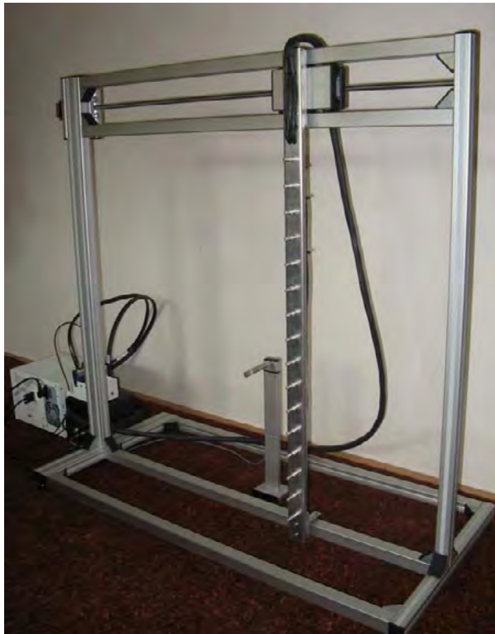
Figure 5.5: Measurement system with linear microphone array and smart microphones.
