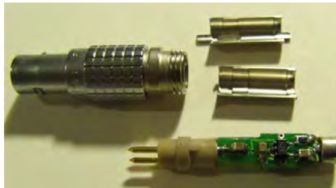
Figure 5.2: Mechanical construction of designed smart microphone.
