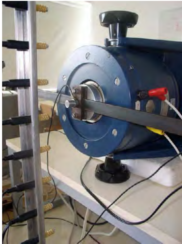
Figure 6.2: Linear microphone array in the acoustic near field of vibrating steel beam excited by shaker.
