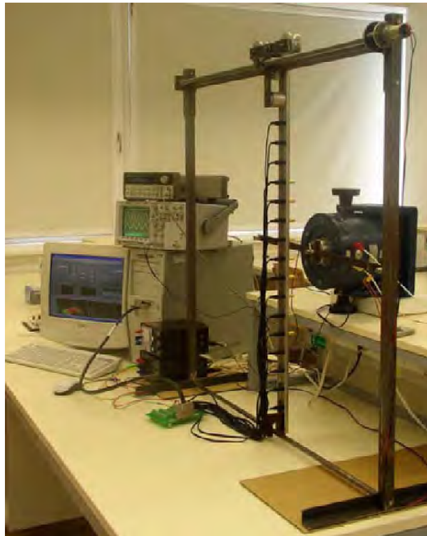
Figure 6.1: Measurement setup for modal analysis of guided-supported steel beam with linear microphone array for acoustic holography method.
