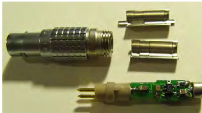
Figure 5.2: Mechanical construction of designed smart microphone.
