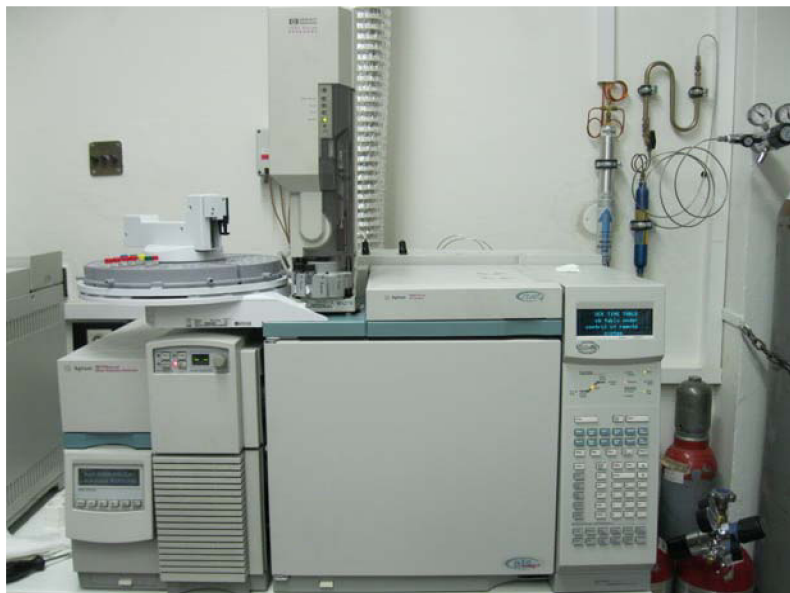
Obrázek 57: Agilent 6890 Series GC System / Agilent 5973 Network Mass Selective Detector
