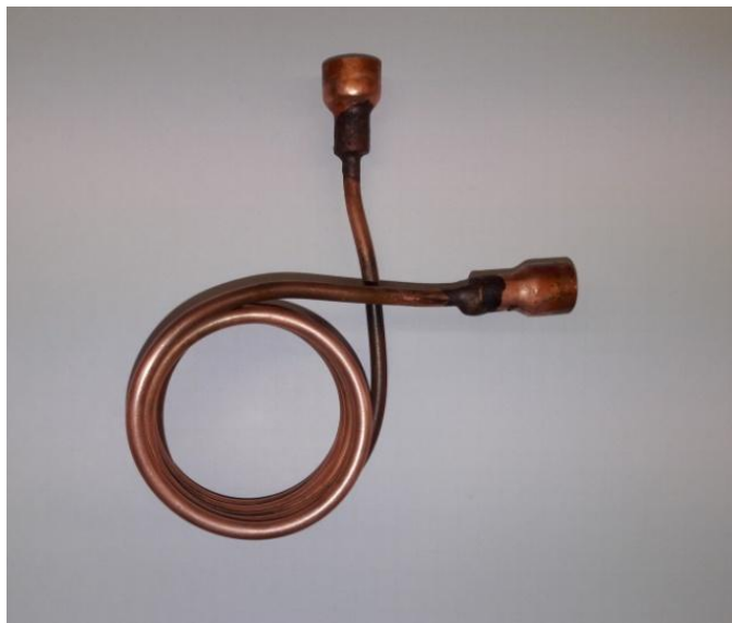
Picture 5.11: Photo of constructed capillary
