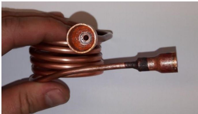
Picture 5.10: Photo of connections of constructed capillary
