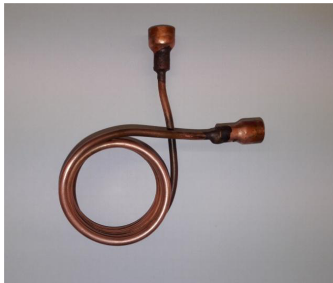
Picture 5.11: Photo of constructed capillary
