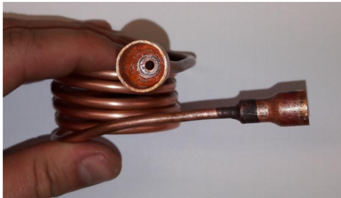
Picture 5.10: Photo of connections of constructed capillary
