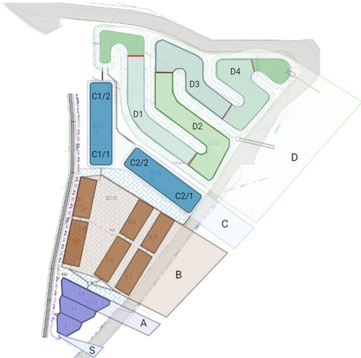
Figure 5. Wetland+ modules. The inlet (S), aeration system including sedimentation (A), permeable reactive barrier remedial system (B), biosorption module (C), and aerobic wetland system (D).
