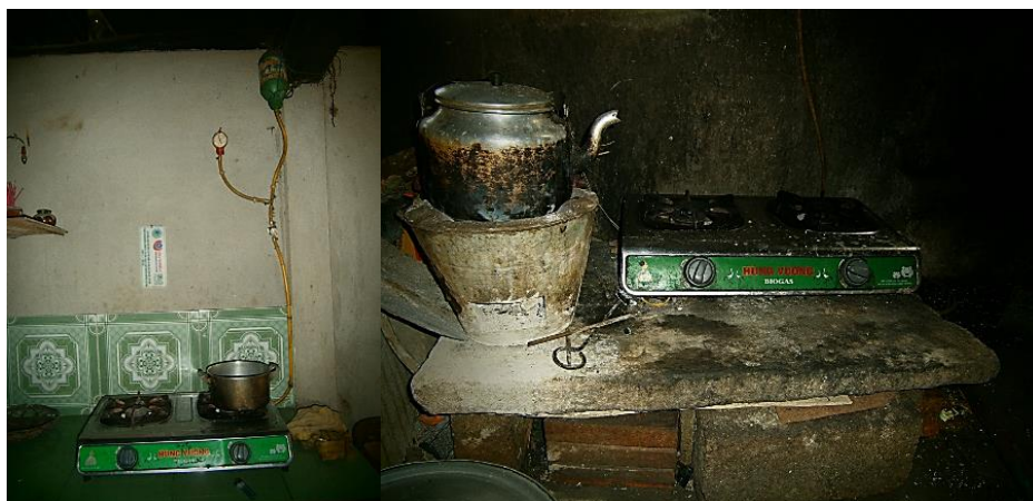
Figure 3 Two-flame biogas cook stoves (left and right) in a Vietnamese rural household.
