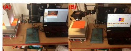
Figure 7. Contact angle of melting PEG droplets on fibrous materials (A) and T-history measurement of sandwich fibrous PEG encapsulations (B).
