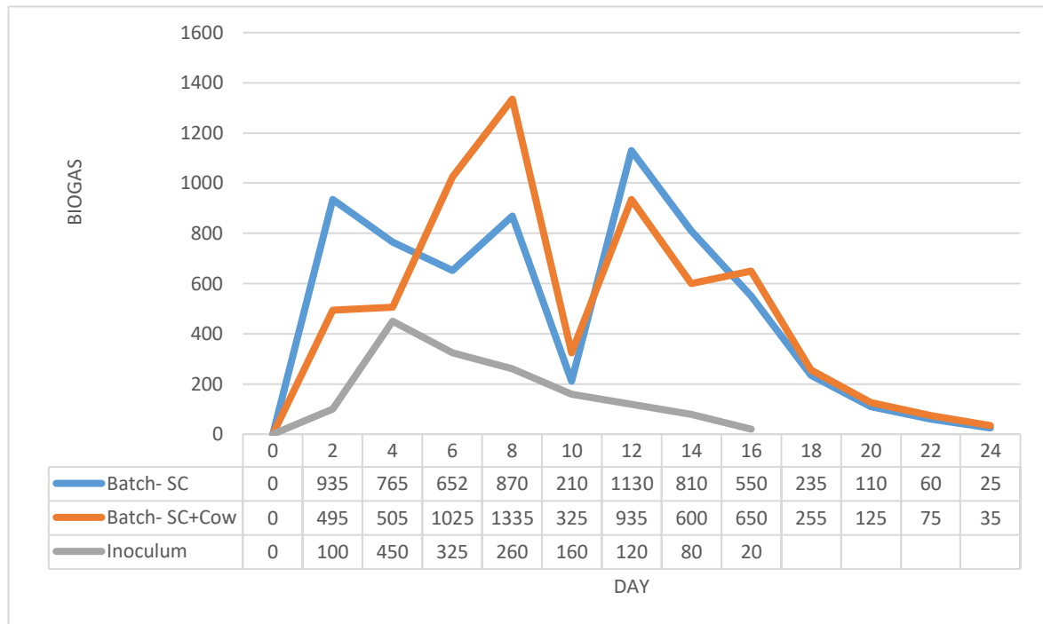
Figure 4. Variation in Biogas production (ml) of Sugarcane bagasse (SB) and co digestion of Sugarcane bagasse and Cow manure, over a period of 24 days.
