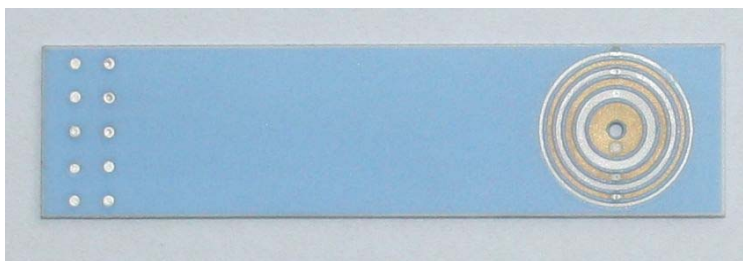
Fig. 14: Array sensor with annular electrodes of the same geometric area
