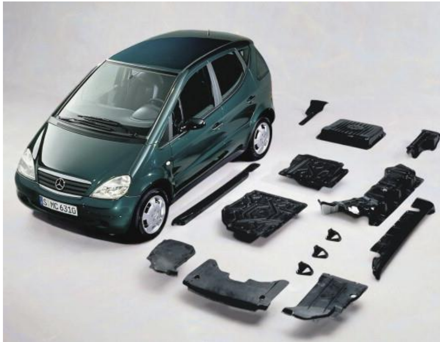
Figure 2.3. Flax/polypropylene underbody components have replaced glass fiber reinforced plastic components in vehicles such as the Mercedes Benz A-Class [61]
