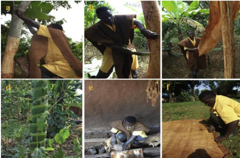
Figure 3.1. Extraction of Barkcloth non-woven natural fabric: (a) Scraping of tree outer layer. (b) Use of local wedged tool to peel off the bark. (c) Peeling of the bark. (d) Covering of the tree stem for environmental sustainability. (e) Pummeling under the shade. (f) Sun drying of the non-woven fabric. [127]
