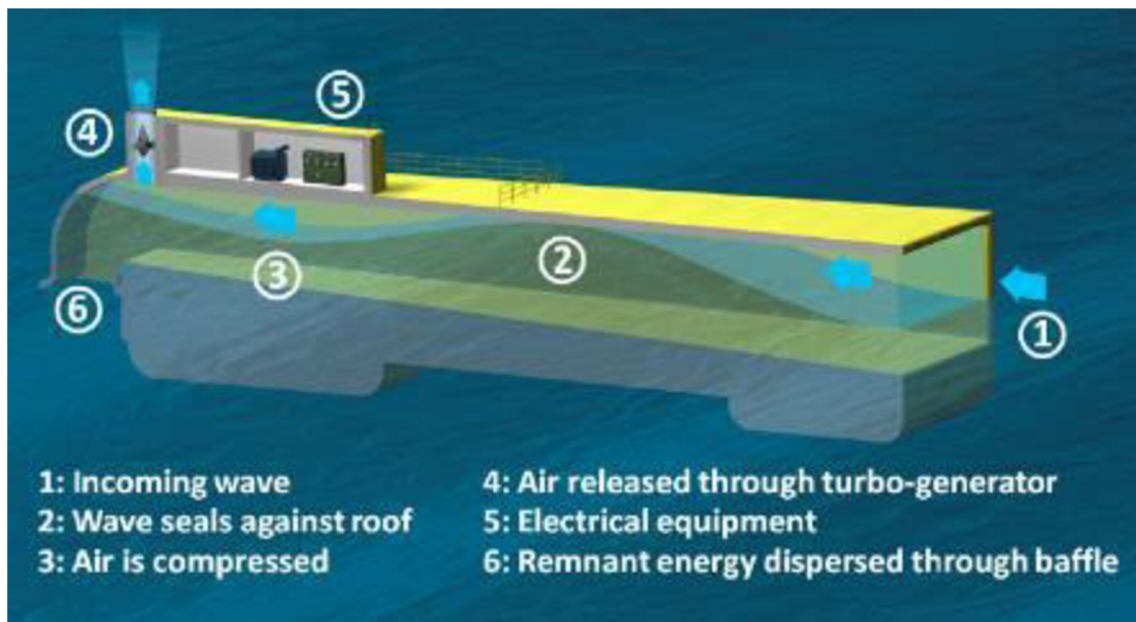
Figure 7. Basic principle of wave generator
