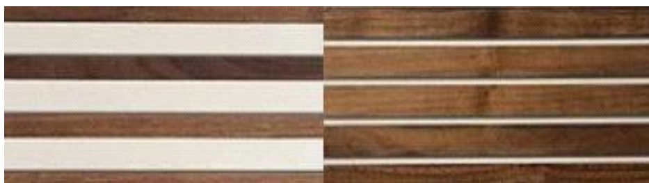
Figure 5: Certain thicknes and width wooden board coating acrylic board surface combinations ( www.fklisty.cz ).
