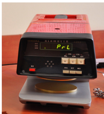
Figure 2-5 Alambeta Working machine for measuring thermal properties [44]
