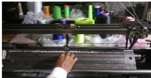
Figure 3-4 Flat knit machine used for the manufacturing of studied samples ( Yarn insertion )
