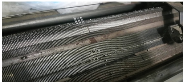
Figure 3-3: Flat knit machine for the manufacturing of the studied samples
