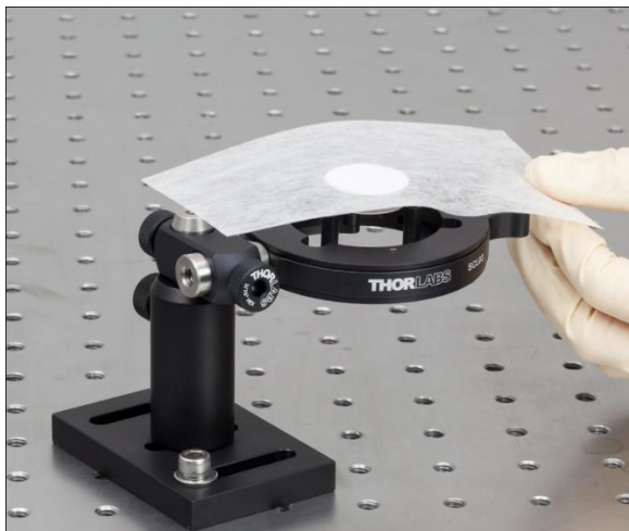
Figure 10: Drag the tissue across the optic [2]
