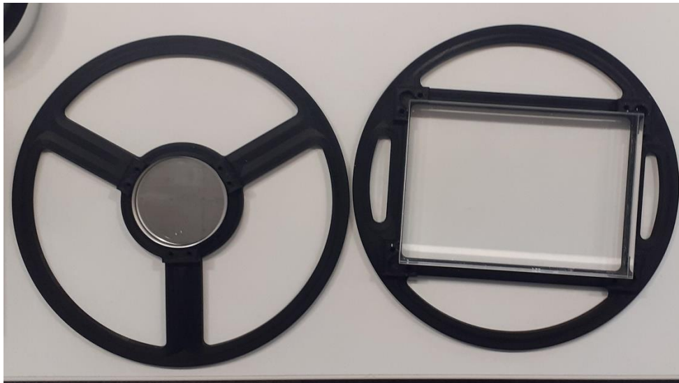
Figure 27: The insert prototype made by 3D printing
