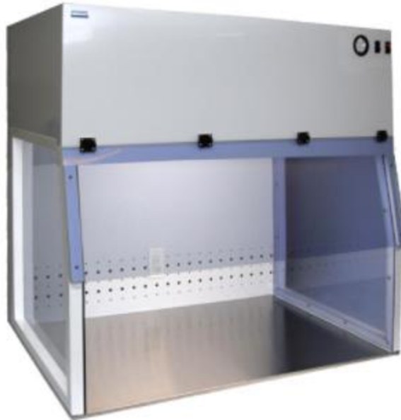
Figure 32: Bench-top Vertical Laminar Flow Hood [9]
