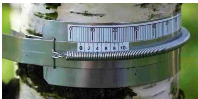
Photo 2: Mechanical dendrometer (EMS Brno, Czech Republic) Source: http://www.usbe.cas.cz/lefr/img/biomasa/obr_02.jpg
