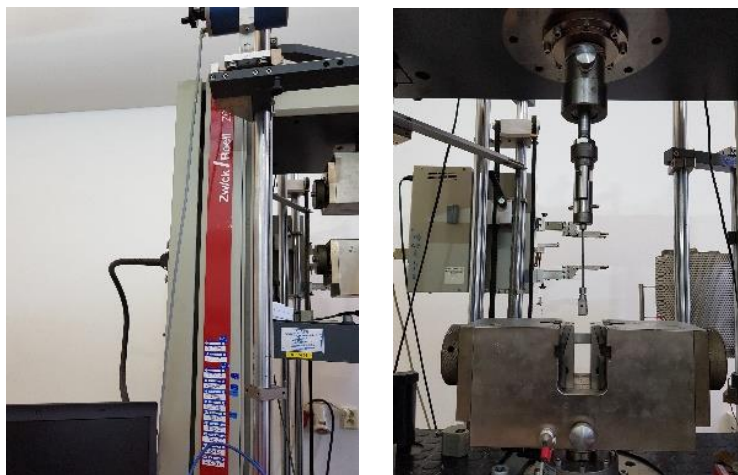
Figure 53: Shows the machine used for the tensile test
