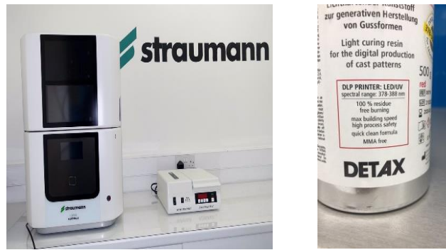
Figure 43: Shows the 3D printer Straumann P series Rapidshape and Detax Freeprint resin for the digital production of the cast pattern (100% residue-free burning)
