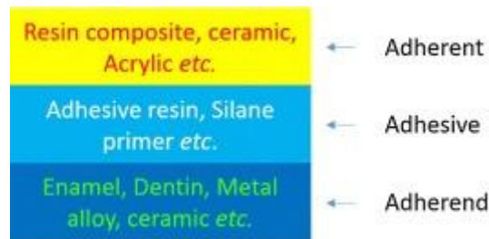
Figure 1: Shows the main process of adhesion in dentistry (Xiao-zhuang Jin et al , 2016)
