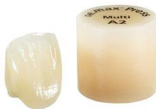
Figure 26: Shows the ingots of lithium disilicate (IPS e.max Press)
