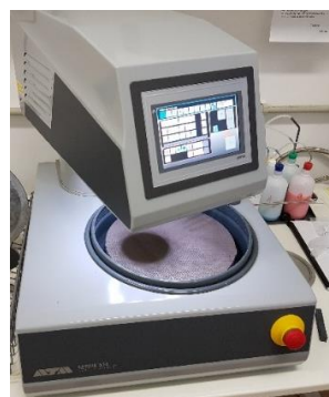
Figure 39: Shows the machine used for the standardization process of the smear layer (Saphir 550)
