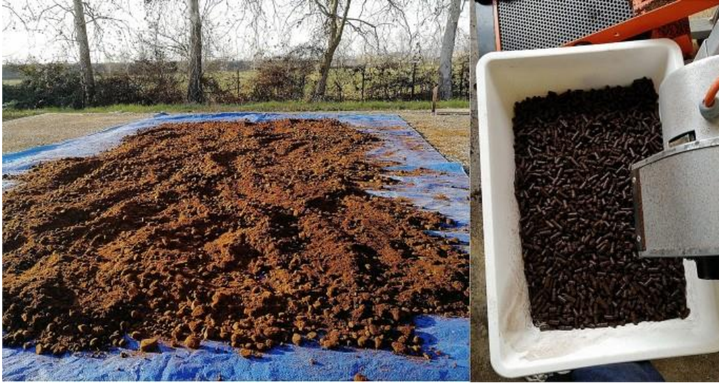
Figure 4. Production of pellets from SCGs
