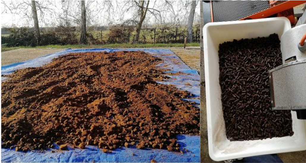
Figure 4. Production of pellets from SCGs
