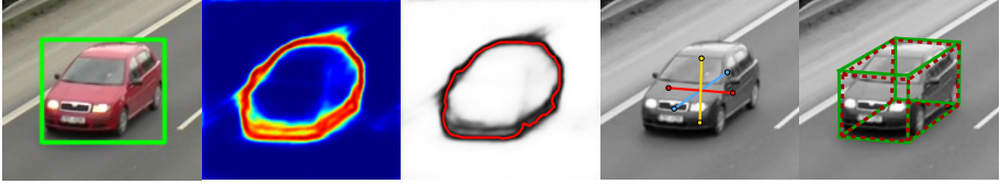
Figure 2.5: Estimation of 3D bounding box. Left to right: image with vehicle 2D bounding box, output of contour object detector [30], our constructed contour, estimated directions towards vanishing points, ground truth (green) and estimated (red) 3D bounding box.
