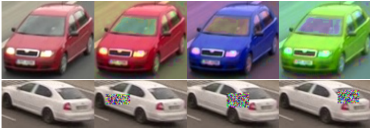
Figure 2.4: Examples of proposed data augmentation techniques. Left most image contains the original cropped image of the vehicle and other images contains augmented versions of the image ( Top – Color , Bottom – ImageDrop ).
