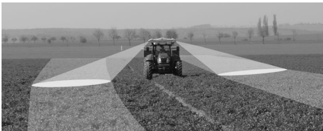
obr.18 Yara N-sensor (BAG 2017)
