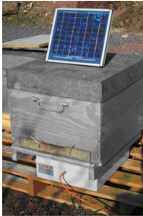
Fig. 4.2: Beehive placed on a weighting system Beewise [5].
