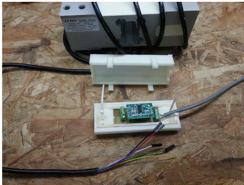
Fig. 5.10: Converter mounted on PCB with 3D printed box.
