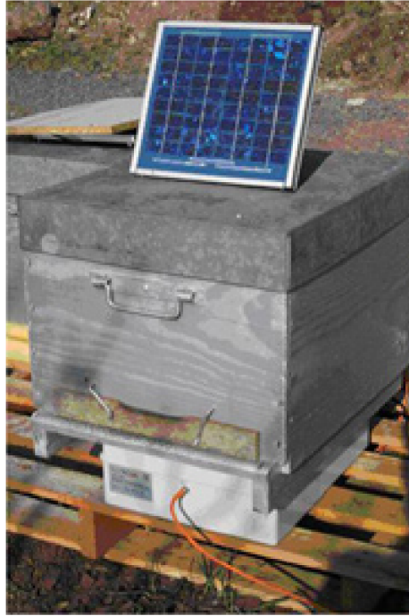
Fig. 4.2: Beehive placed on a weighting system Beewise [5].
