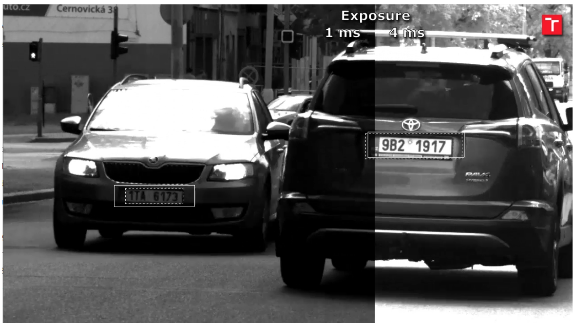
Figure 4.20: A real traffic situation captured by camera prototype by Nosko et al. [42] with embedded licence plate detector [40] (working on LDR images only); Image is obtained from presentation for projects EMC2 and Almarvi. The dash type of rectangle marks, in which source exposition the licence plate was found.
