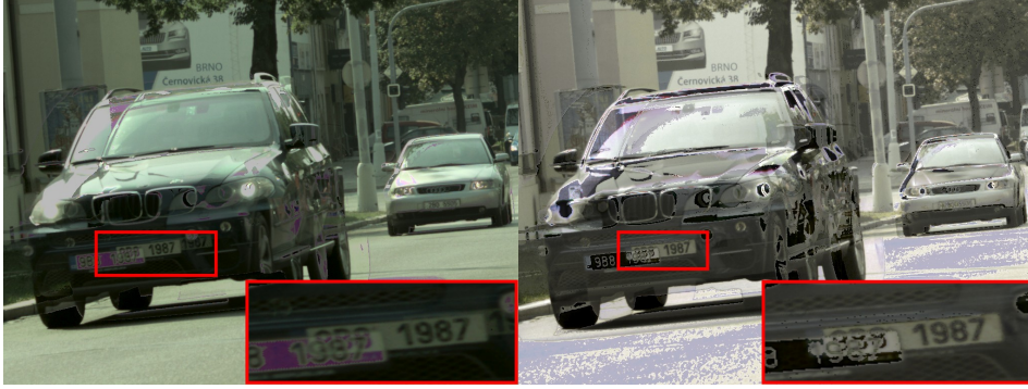
Figure 4.6: Sample outputs of related deghosting algorithms by Pece et al. [44] (left) and Min et al. [35] (right) on the scene from Figure 4.1. Our experiments revealed that listed algorithms should be successful only on images with convenient histogram distribution.
