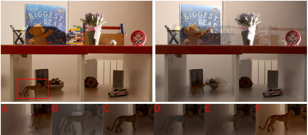
Figure 4.9: Output of the proposed HDR ghost-free merging method for Complex Scene 1 of dataset [23] (left). Ghosted HDR image is shown on the right. Previews of various algorithm results are shown at the bottom. No de-ghosting (A), Silk et al. [52] (B), Sen et al. [50] (C), Photoshop (D), Photomatix (E) and proposed algorithm (F). The previews A to E are published as a part of a Karaduzovic dataset [23].
