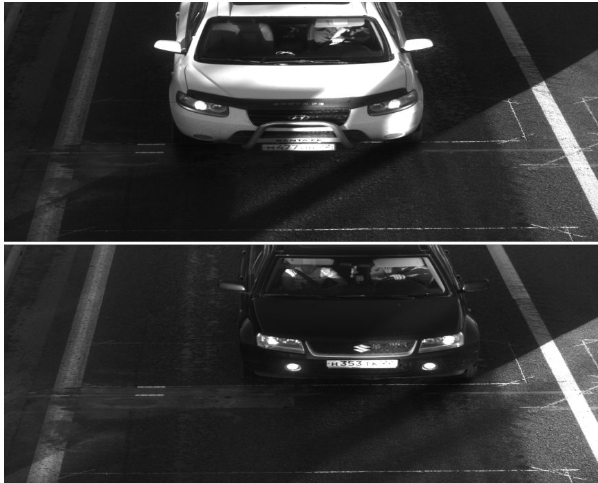
Figure 4.16: A real photos taken from section speed cameras (without HDR mode). The actual position of the sun makes the licence plate unreadable. Images obtained from Camea spol. s r.o. ( www.camea.cz ).
