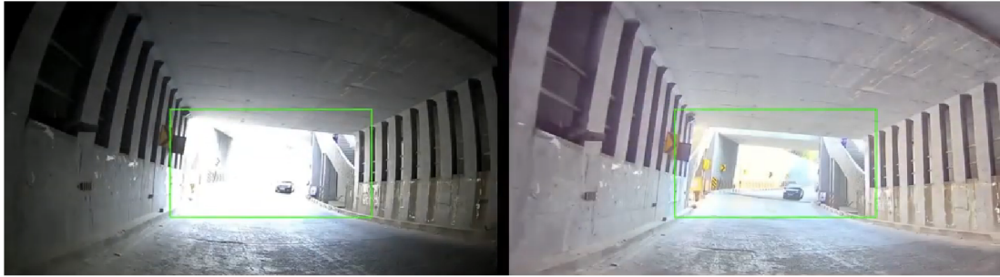
Figure 4.17: Illustrative comparison of non-HDR mode (left) and HDR (right) on an automotive application. Image was taken by Hyperyon camera and obtained from https://www.e-consystems.com .
