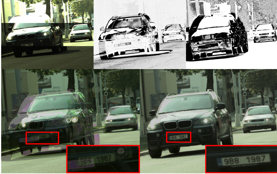
Figure 4.1: Figure obtained from real application of proposed ghost-free algorithm - traffic monitoring system with licence plate detection, which demonstrates the contribution of proposed method. Top left - stripes of original images with a significant car motion. Top middle and top right - Images representing coefficients used for the HDR merging ( certainty maps , see Section 4.1). Bottom left - ghosted HDR image. Bottom right - HDR image merged using proposed method.
