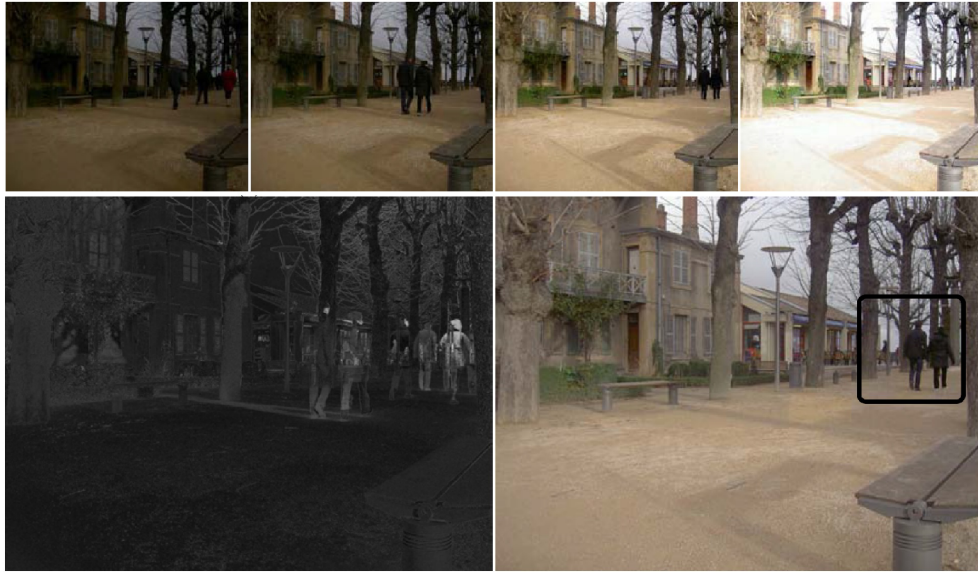
Figure 2.6: The Figure shows the results of variance based deghosting method by Jacobs et al. [18]. The variance map (bottom left) is obtained from the image sequence (upper row) and used to generate the HDR image (bottom right). Figure obtained from [18].
