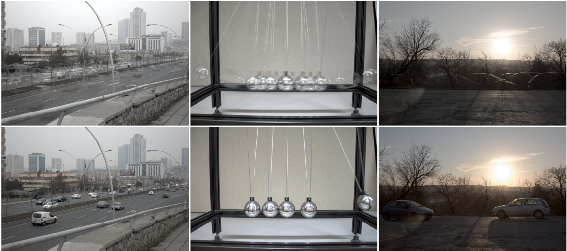
Figure 4.4: Ghosted HDRs (top line) and HDRs merged using proposed ghost-free method (bottom line) on sequences „Fast cars“ [59] (left), „105“ [60] (middle) and „117“ [60] (right). Datasets contains 9 LDR (Low Dynamic Range) images.
