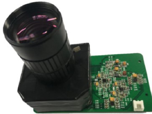
Figure 3.19: The hardware platform of the camera by Tang et al. [56]. Image retrieved from [56].
