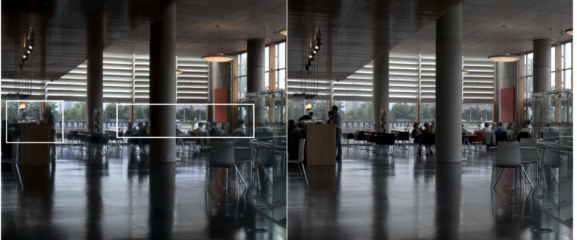
Figure 4.10: Figure shows scene „Cafe“ from Tursun’s [59] dataset processed with Sen [50](top) and the proposed ghost-free algorithm(bottom). Sen [50] produce a heavily blurred image, which precludes the HDR-VDP metric [33]; moreover, the de-ghosting method fails (see marked areas, where objects are shadowed and blurred).
