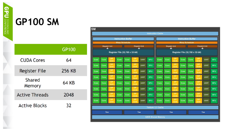
Figure 3.2: Schematics of SMP from nVidia Pascal GPU. Image retrieved from https://wccfttech.com/nvidia-pascal-specs/ .
