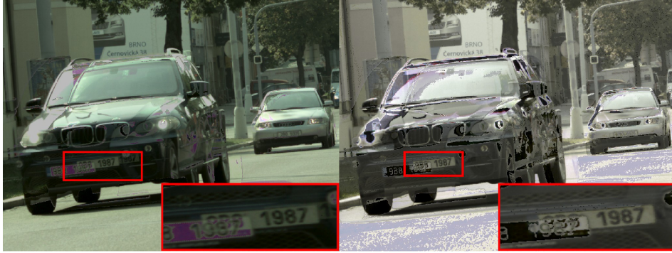
Figure 4.6: Sample outputs of related deghosting algorithms by Pece et al. [44] (left) and Min et al. [35] (right) on the scene from Figure 4.1. Our experiments revealed that listed algorithms should be successful only on images with convenient histogram distribution.
