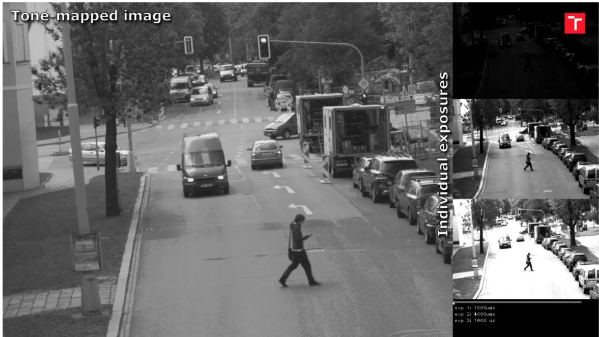
Figure 4.14: A Graphic output of HDR camera prototype from Nosko et al. [42]. The image is tonemapped by Reinhard et al. [47] operator. The source image sequence is shown in the right column.
