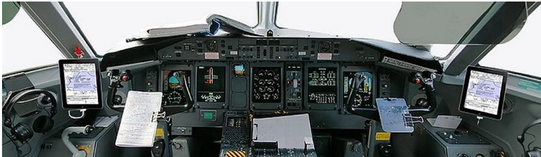
Figure 2.1: Apple iPad as an EFB device in an airplane cockpit [21].
