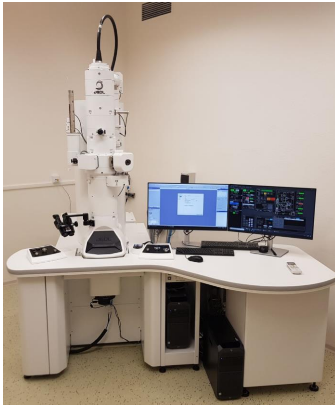
Figure 4: Transmission electron microscope TEM JEM-1400 JEOL, located at the Laboratory of Electron Microscopy in České Budějovice (BIOLOGICKÉ CENTRUM AV ČR, v. v. I. | Mikroskopy a Počítače pro Zpracování Dat, n.d.).
