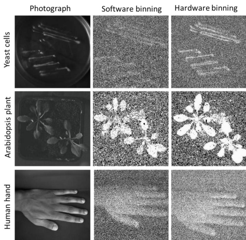
**Figure 17:** Two-dimensional imaging of spontaneous ultra-weak photon emission from *Saccharomyces cerevisiae* (A), *Arabidopsis thaliana* (B) and human hand (C) measured with software and hardware binning mode of  $4 \times 4$  and accumulation time of 30 min.
