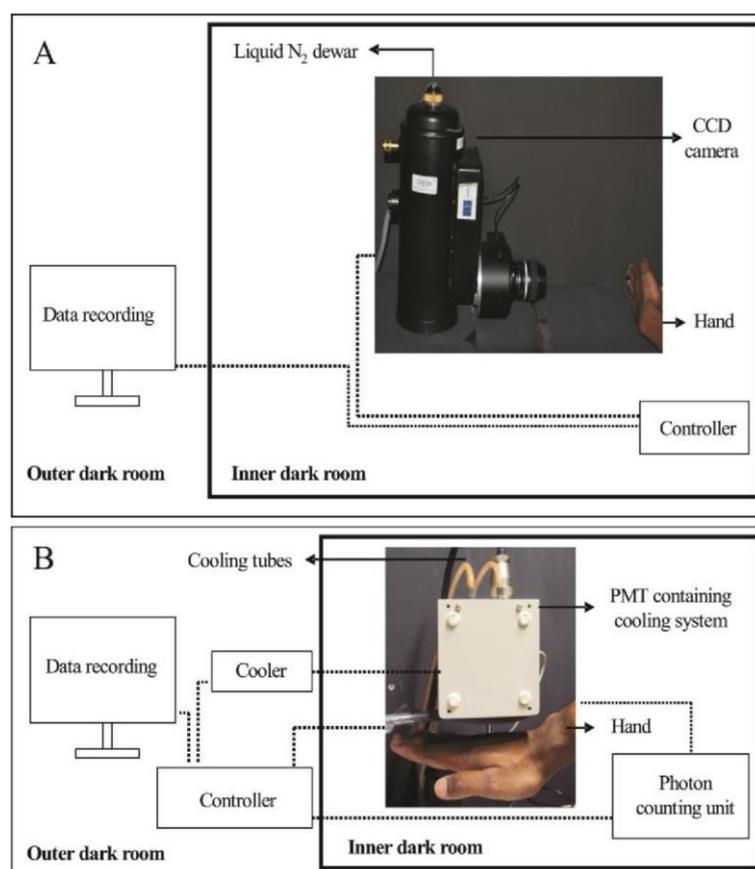
**Scheme V:** Schematic illustration of the experimental setup for detection of two-dimensional (A) and one-dimensional (B) ultra-weak photon emission. Two-dimensional ultra-weak photon emission was detected by CCD camera positioned horizontally. One dimensional ultra-weak photon emission was detected by PMT positioned vertically. The distance between the sample and PMT window varied based on the sample measured [Fig. 1, Article II].
