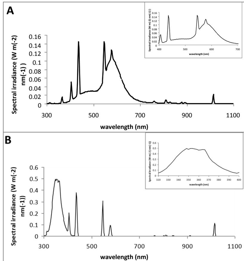
**Figure 11:** Spectra of visible light (A) and UVA radiation (B) source was measured by employing Spectral Radiometer; LI-COR LI-1800 (LI-COR Biosciences, St. John's Innovation, Cambridge, UK).
