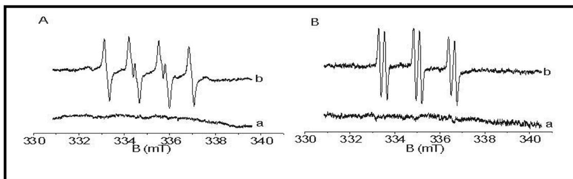
**Figure 10:** Detection of  $O_2^{\bullet -}$  (A) and  $HO^{\bullet}$  (B) by EPR spin-trapping spectroscopy in the absence (a) and presence (b) of reaction mixture forming ROS (Fig. 5, Article II).
