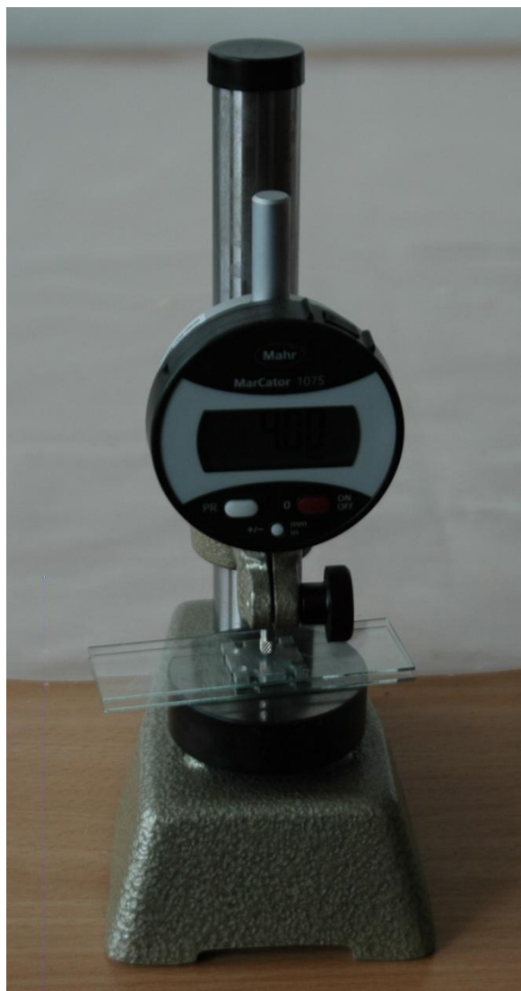
Figure 40 Device for measuring of wall thickness. Tissue is placed between two glasses and the wall thickness is measured by a drift meter.
