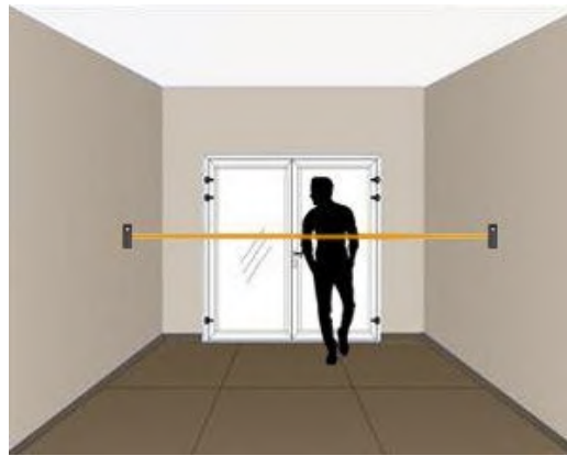
Figure 2.1: Infrared/laser barrier sensor for counting people passing through. (Source: [42].)
