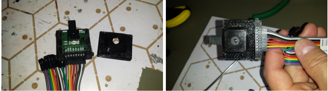
Figure 3.9: 3D-printed case for the Lepton 3.5 in a breakout board.
