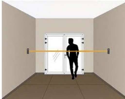
Figure 2.1: Infrared/laser barrier sensor for counting people passing through. (Source: [42].)
