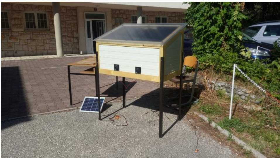
Figure 15. Solar dryer at University of Mostar
