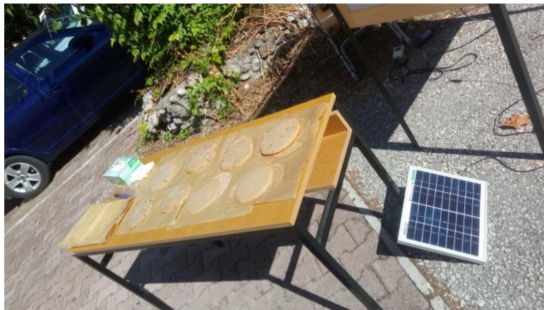
Figure 17. Open sun drying on a desk at University of Mostar
