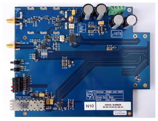
Fig. A.5: Top view of the ADC Subsystem module
