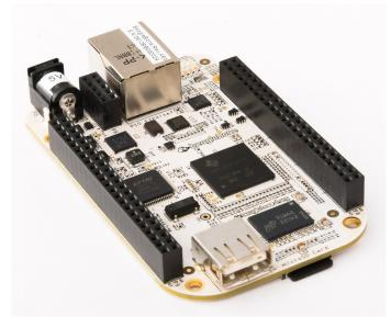
Fig. 2.22: BeagleBone microprocessor module
