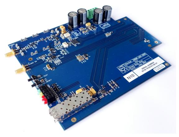
Fig. A.4: Perspective view of the ADC Subsystem module
