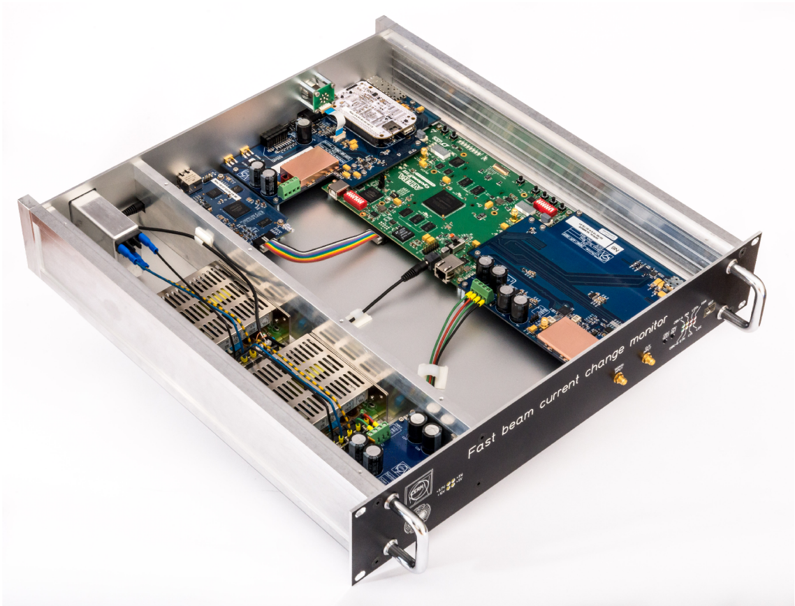
Fig. A.14: Perspective view of the FBCCM device without top panel
