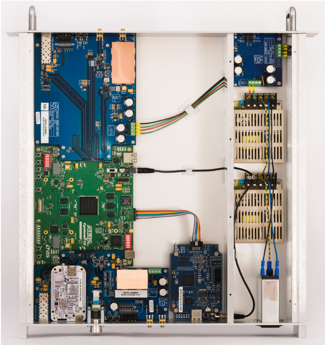
Fig. A.15: Top view of the FBCCM device without top panel
