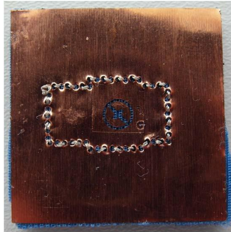
Figure 53 Photograph of the version 1 antenna for the ISM band 25 GHz; manufactured from copper foil.
