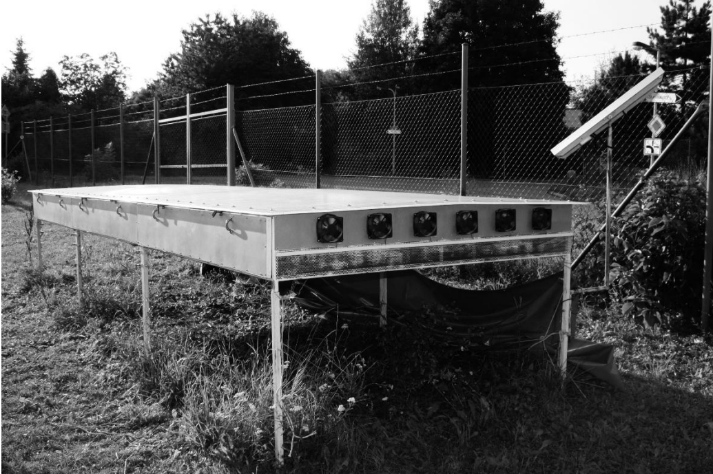
Figure 3.4 General view of Double-pass solar drier.
