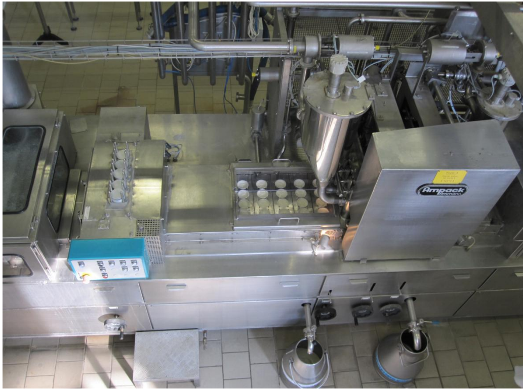
Appendix 6: Filling of the yogurts in dairy plant Bohušovice (photo Kamila Nováková, 2011)
