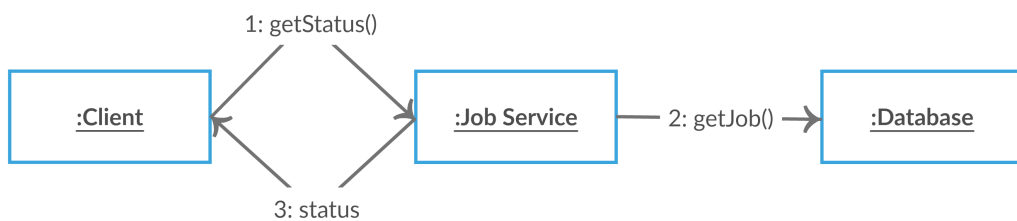
Figure 3.6: Collaboration diagram of a job status retrieval
