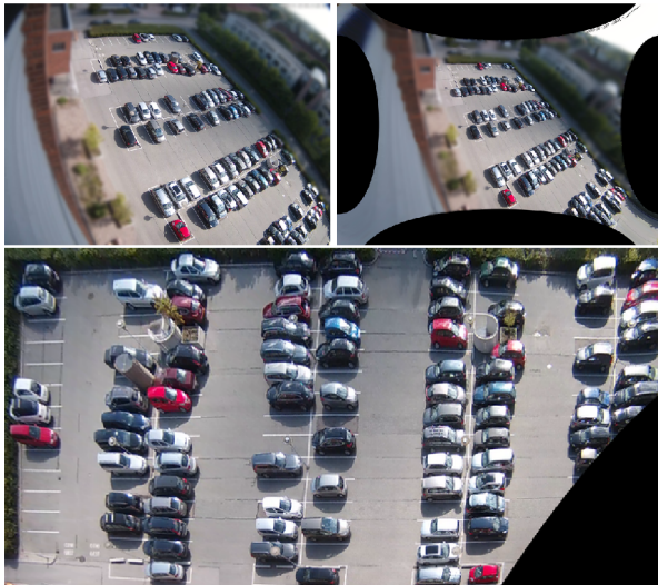
Figure 3: Original image, image after removal of distortion and image after removal of perspective
