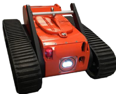
Obr 6 TML: Glimpse Remote Inspection Robot [11]
