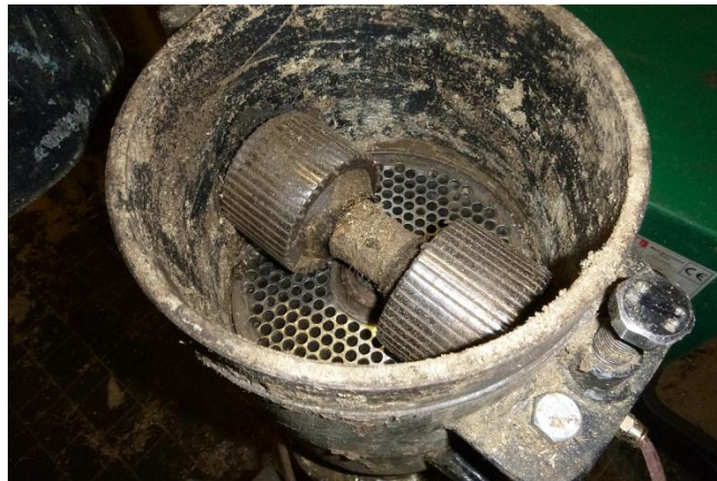
Figure 6.: Detail of flat die with rollers
