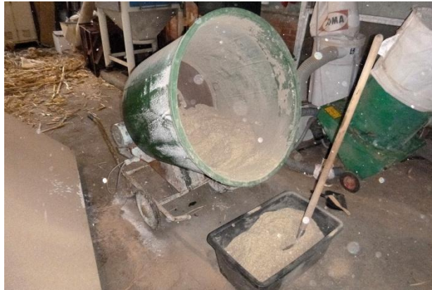
Figure 4.: Universal mixer with sample
